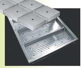
The magnetic area is made of a modular polar plate machined from a solid block, and is fixed with special high resistance screws to the main body which is also built in a monoblock construction. The area with coils and the electric circuits is protected mechanically, in addition to the insulation given by the high resistance resin. The lean design with no other fixing
