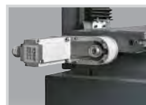
Application example as feed unit of the X-axis
