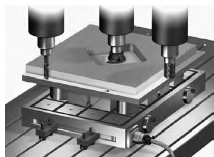
Figure 8.7D - Tilting, roughing, release of stress and finishing of second surface
