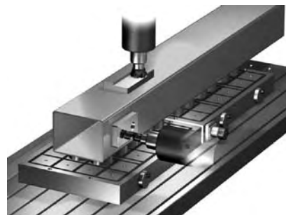
Figure 8.7F - Butting and drilling of tubular sections
